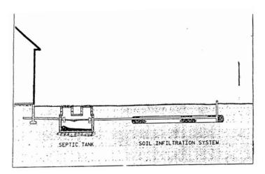
A septic tank is typically the first component of a septic system. A system can be as simple as a septic tank and drainfield or include any number of add-ons, such as an effluent filter, aeration tank, sand filter, pump/siphon chamber or sand mound.
