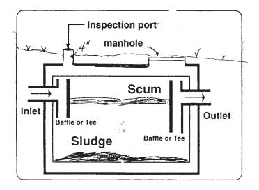
A septic tank looks like the illustration above. The size of the tank depends upon the number of bedrooms in the house, not the number of people or plumbing fixtures. The sizes range from 750 gallons on up and may be configured as one or two septic tanks. Having two septic tanks (or a two compartment septic tank) increases detention time of the waste water, which helps to further reduce the suspended solids that could flow into the drainfield.
